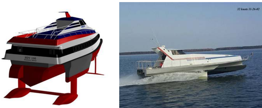
Fig. 8. Blended-wing-body configuration sketch and picture of the HDV-100 technology demonstrator (shown here at low speed)
